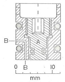
Fig. 2. An O-ring plug for the optical cell
